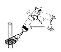
Hold the applicator at an angle of 30° to 45° to the object. This will direct paint more to target area.
