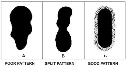
Dirty, worn, or damaged nozzle. Clean or replace.
