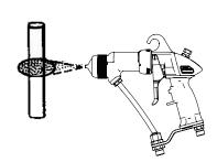
Increase the applicator to target distance to approximately 10-12-inches. This will decrease the speed of the paint particles in the vicinity of the target.
