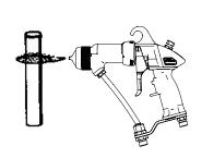
Adjust the fan for a pattern width slightly wider than the object. This allows some coating material to start around the sides of the object.
