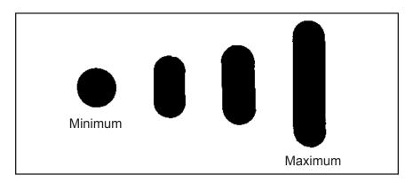
The size of the object being coated is the determining factor in adjusting the fan pattern; the larger the object, the larger the required fan pattern. Fan control of the Ransburg Vector/Solo applicators is accomplished by rotating the adjusting knob located at the rear of the applicator. Fan width can be set for approximately a 3-inch width (minimum) to approximately a 14-inch (maximum). Fan widths and overall pattern appearances are illustrated.
