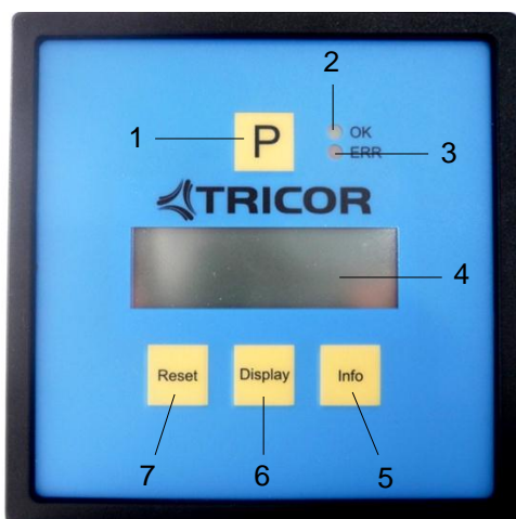
Fig. 5: Operating Elements of TCE80xx-S
