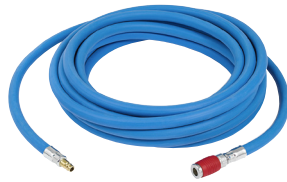
High-quality air hose for connecting spray guns and breathing protection systems 9 mm inner diameter, 10 m long, with quick coupling and nipple, antistatic, conductive, free of substances causing coating flaws, 20 bar pressure-resistant, high bursting safety. Art. No. 53090
