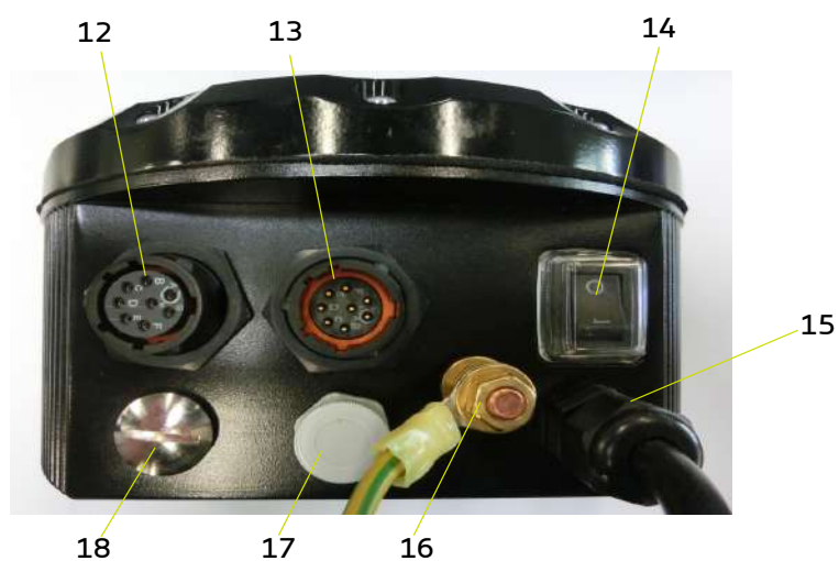
Side face of the GNM 6080 control module
