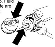
**3.** Check the Fluid Nozzle is secure & leak free.
