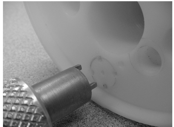
Face of Fitting Flush with Manifold
