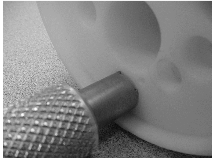
Tighten Fitting Into Manifold
