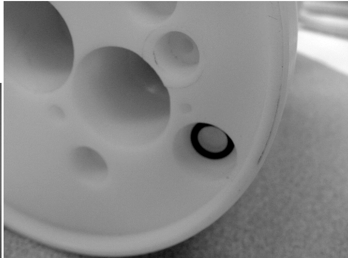
Install O-Ring Into Manifold
