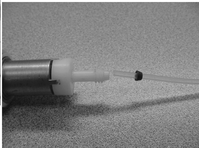
Slide Ferrule Onto Tubing
