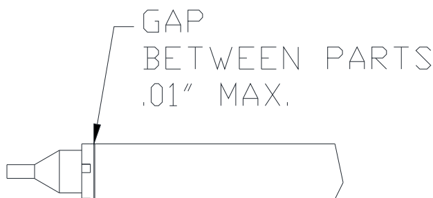
Figure 31: Fluid Tip/Tube Gap
