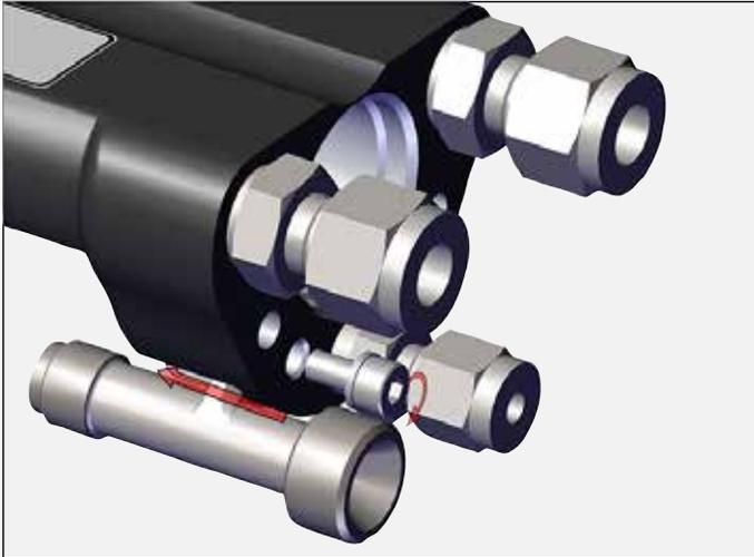
6. Install cascade housing onto piston housing.
