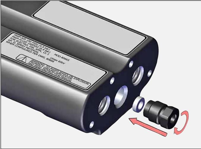
5. Install fluid inlet fitting.
