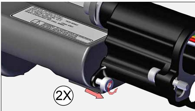
12. Remove internal housing screws.
