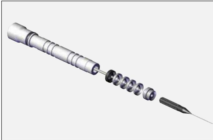
7. Insert packing tube onto shaft. Wipe excess grease over front parts and outside of packing tube.
