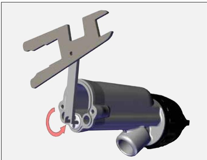
6. Insert 4 parts on front of shaft.
