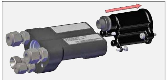
14. Remove needle packing nut and packing.
