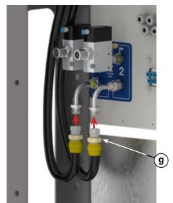
8. Remove and discard one of the air fitting plugs (h) from the Y splitter push-in fitting. The second air feed is reserved for future or optional peripheral accessories.
