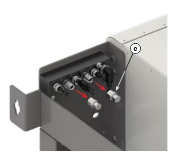
6. Attach the ErgoFlex hoses (f) to the fittings and tighten.
