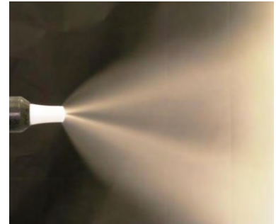
too much electrode rinsing air
