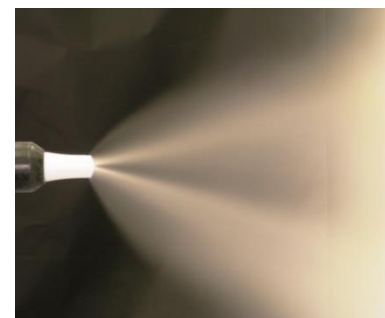
too much electrode rinsing air
