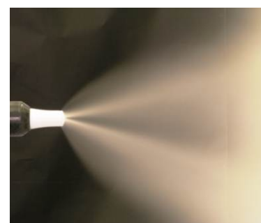
too much electrode rinsing air
