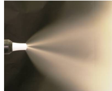
too much electrode rinsing air
