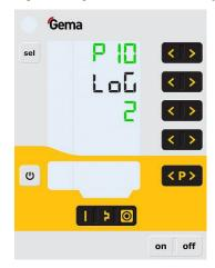
The device can export log reports of the program run to an SD card for test purposes and for finding defects.
