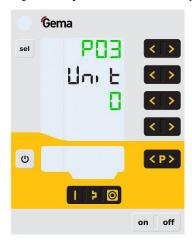
This parameter is used to determine the measuring unit for all airs (total air and electrode rinsing air). If the parameter is set to **1** (**scfm**), then all air values are shown in this measuring unit. These lines are displayed in **blue**.
