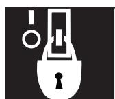
**DE-ENERGIZE, DEPRESSURIZE, DISCONNECT AND LOCK OUT ALL POWER SOURCES DURING MAINTENANCE**
