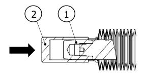
Screw Item No. 2 (assembly spigot) onto the piston shaft
