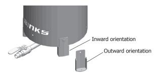
Legs can be oriented either inward or outward to provide flexibility in mounting.
