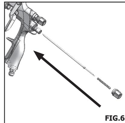
**Tighten to complete stop. Do not over tighten!**
