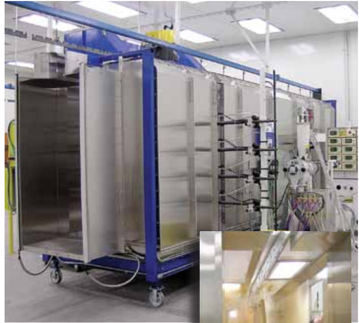
Custom designed booth openings such as operator shields and touch-up windows create a safe and efficient working environment.
