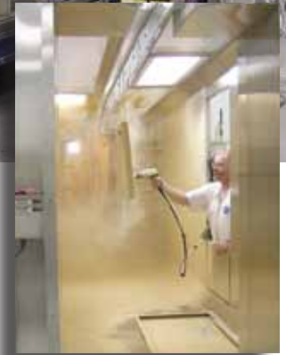
Custom designed booth openings such as operator shields and touch-up windows create a safe and efficient working environment.
