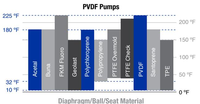
The maximum temperature listed is based on the ATEX standard for T4 temperature classification. If you are operating in a non-explosive environment, FKM fluororelastomer's maximum fluid temperature in aluminum or stainless steel pumps is 320°F (160°C). Actual pump performance may be affected by prolonged usage at temperature.
