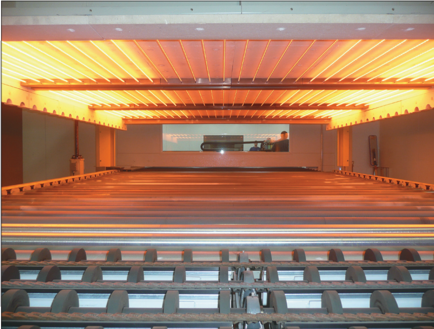
Lamp Lane Zoning Dryer is in "up" (access) position
