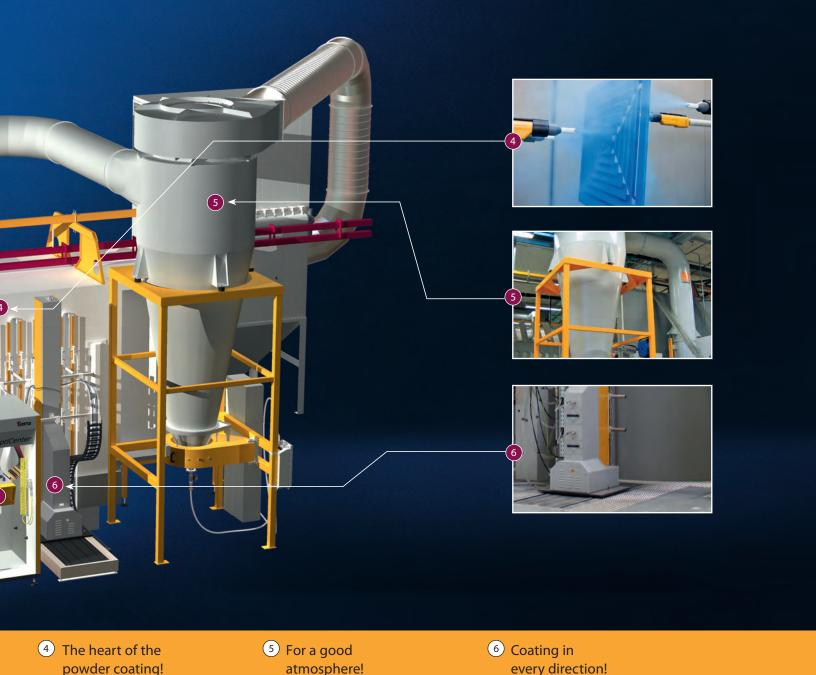
With high transfer efficiency, uniform powder application and optimal penetration into any geometry, the OptiFlex Series powder guns constitute the heart of the powder coating process. The colorchange-friendly construction, which utilizes very few components that are subject to wear is an additional plus. The excellent ergonomics and the lightweight design of the OptiFlex manual guns, guarantees fatigue-free coating.
