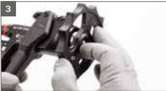
Finally, unscrew the paint nozzle using the ring wrench integrated in the universal wrench.
