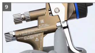
9 Grease visible part of air piston rod
